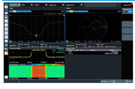
MultiView provides a convenient overview of all active R&S®ZNL modes. Here you see the combination of spectrum analyzer and network analyzer. In this view, all modes can be updated sequentially.
