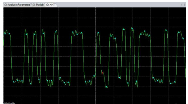
Errored symbol (red dot) in Measurement vs. Time plot.
